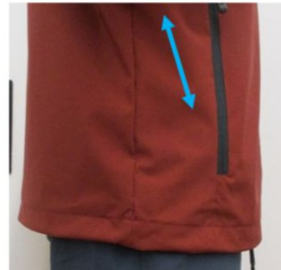
( C-2) slight dragline at front panel under armhole joint seam
